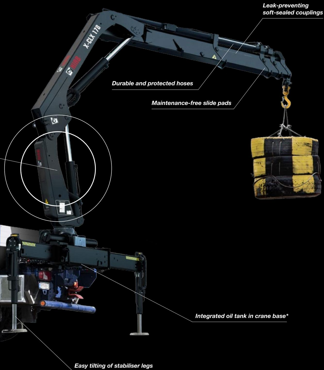
*Leak-preventing soft-sealed couplings*
