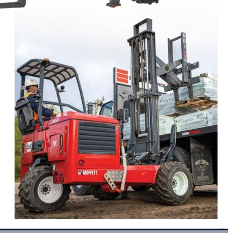
PATENTED MOFFETT *LIFT ASSIST®* ARMS ALLOW THE PANTOGRAPH OPERATOR TO SAFELY REACH CROSS-DECK AND PICK UP FULL CAPACITY, EVEN DOUBLE-STACKED
