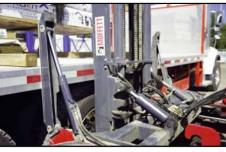
Nylon wear pads on the Lift Assist Arms maximize the contact area and minimize contact pressure on the bed rails providing optimum lift assistance.
