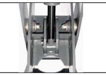
The Central Pivot Shafts in the Pantograph have thrust pads that are fully adjustable with grease zerks to provide wear resistance, ensure smooth operation, and long life.
