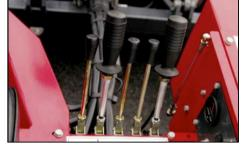
The Carriage Travel/Pantograph functions and the Stabilizer/Lift Assist functions are electro-hydraulically sequenced to ensure safe and precise load handling.
