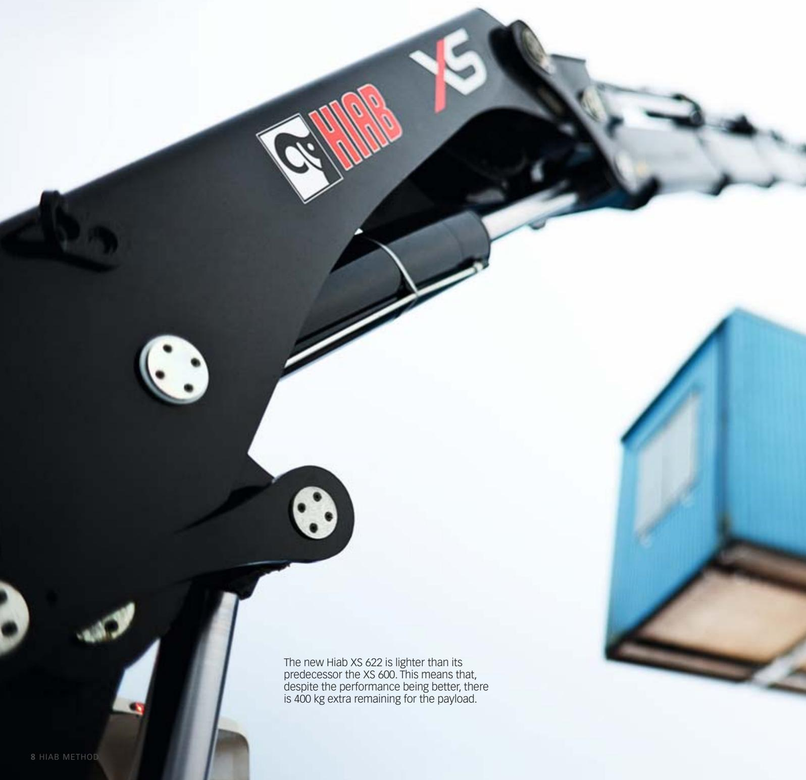
The new Hiab XS 622 is lighter than its predecessor the XS 600. This means that, despite the performance being better, there is 400 kg extra remaining for the payload.
