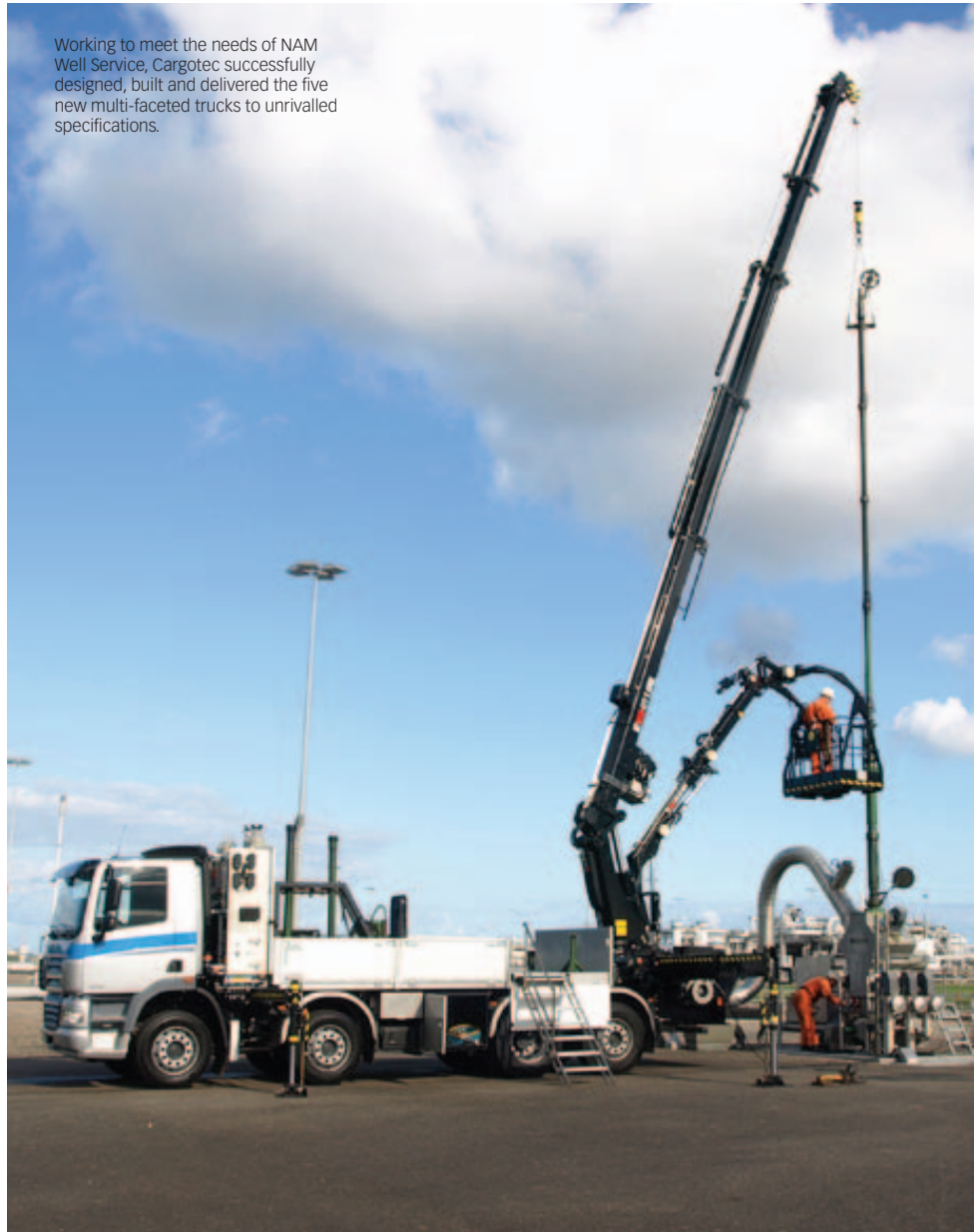
The remote radio control system is ATEX certified and enables the operator in the MEWP to control the crane and installation process on top of the Xmas tree with extreme precision.
