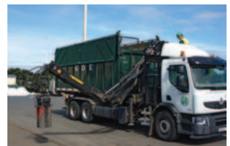
Thanks to careful planning, the driver does not have to leave the vehicle to reach the control platform of his Hiab Jonsered crane.
