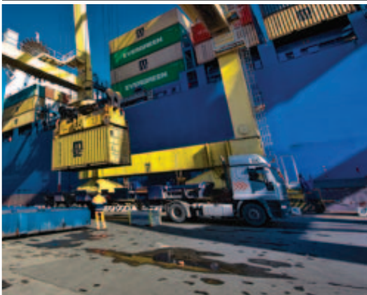
A Kalmar ship-to-shore crane places the container onto the cargo vessel.
