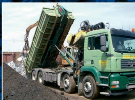
Austria. The combination of the MULTILIFT LHZ hooklift and JONSERED 2640Z recycling crane is the most commonly used combination in Austria.
