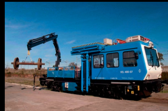
VEL 400 go-devil, a self-powered railroad servicing car, equipped with a HIAB XS 122 E4 HiPro loader crane.
