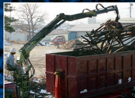
Japan. The versatile LOGLIFT crane and MULTILIFT hooklift combination with a 10-tonne capacity can be used to collect and transport different kinds of waste loads.
