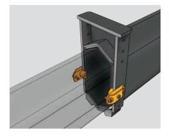
Side supports for stability Side supports fitted on each boom extension stabilize the boom latera
